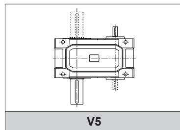
Gearboxes of sizes HDP 60... HDP 90 in mounting position V5 are supplied with upper bearings (not immersed in oil) lubricated with grease and do not require periodic maintenance.
