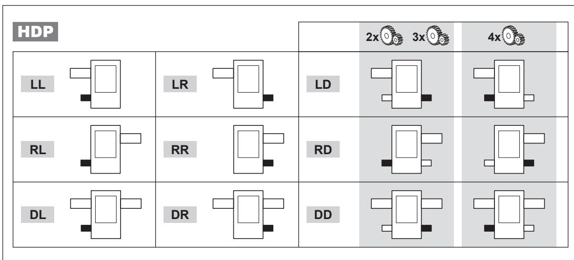
If an overhung load is applied to both shaft ends, contact Bonfiglioli Riduttori's Technical Service for advise.
